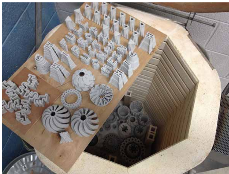
Fig. 14. Loading an electric kiln
